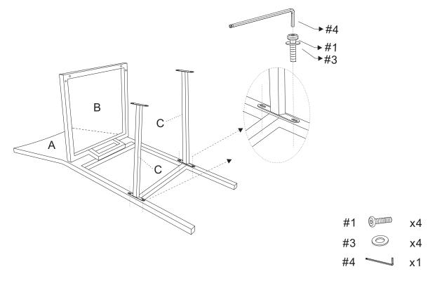
Step 3.Attach front leg (part #D) to assembled parts (part #A,B&C) using short bolts (part #1), washers (part #3) and allen key (part #4).
