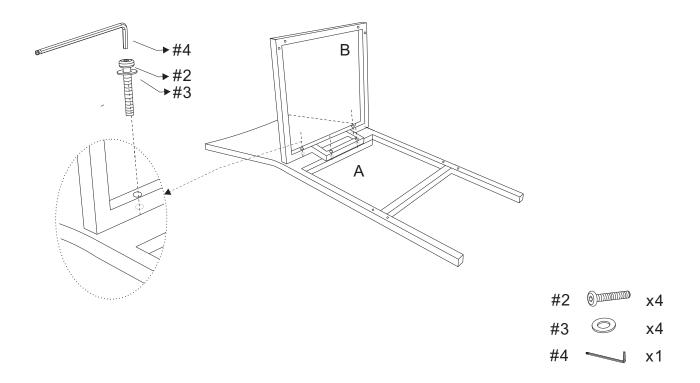
Step 2.Attach stretchers (part #C) to back panel (part #A) using short bolts (part #1), washers (part #3) and allen key (part #4).
